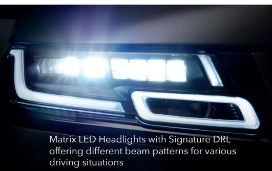
Matrix LED Headlights with Signature DRL offering different beam patterns for various driving situations
