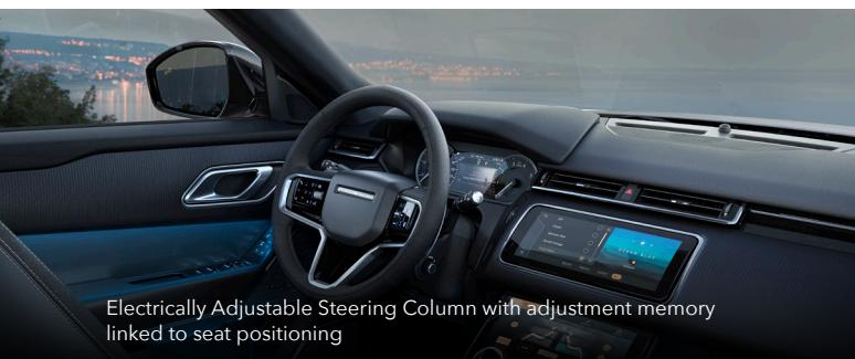
Electrically Adjustable Steering Column with adjustment memory linked to seat positioning
